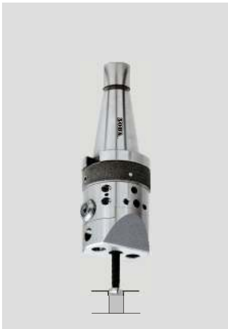
Making of a very small diameter bore (carriage locked) Tool shaped to requirements
