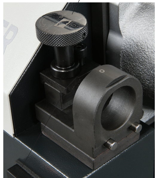
Stopper for flute end point (blade)
