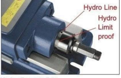
Hydraulic controller: provide stable pressure, Hydro indexer. Protect the hydro system. Hydro limit proof reference scale. Screw shaft broken proof.
