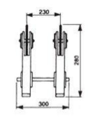
The stand is specifically designed to improve accuracy and longer life for grinding. It is finished with cast iron and fine through hardened to HRC 55°.
