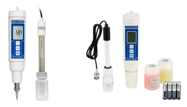
PCE-PH20easy-to-use water analysis meter for pH determination / External pH electrode / Recalibratable / Waterproof (IP 67)
