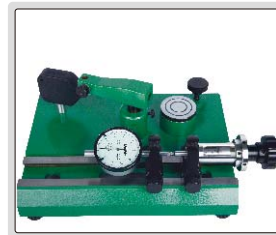
inspect accuracy of dial indicators (range 0-25mm)
