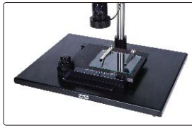
X-Y glass stage (optional) (X-Y travel: 74×60mm)
