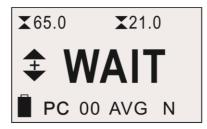
If "I.DLY" is shown on the display, the force gauge will wait until the set minimum time has elapsed.
