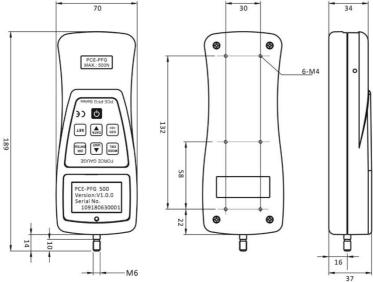
Dimensions for models with external measuring cell
