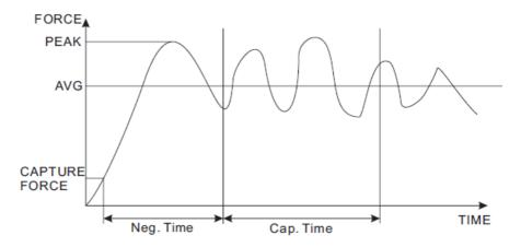
**MOD2:** This function calculates the average above the set smallest measured value. When the measured value falls below the set smallest measured value again, the measurement is finished. This measuring procedure is possible over a period of 10 minutes.
