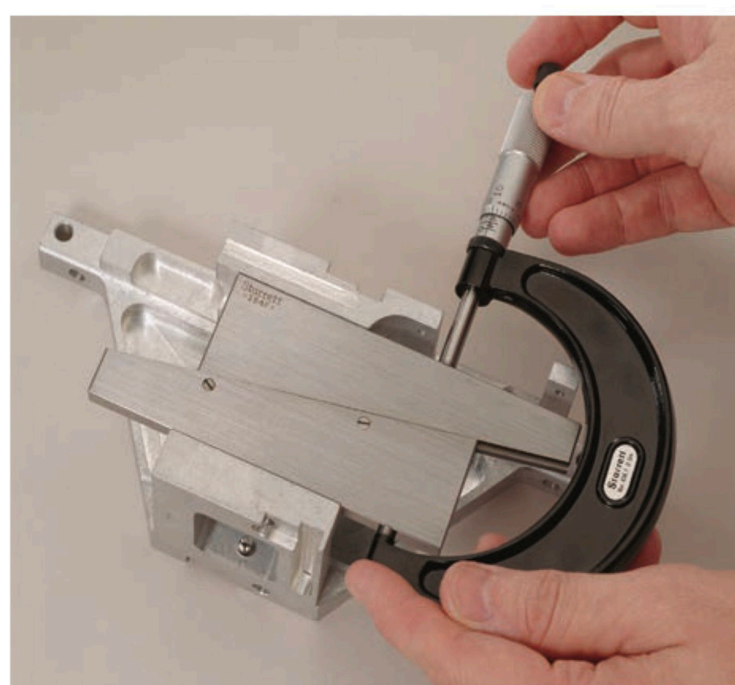
Checking inside measurement of slot with parallel and outside micrometer
