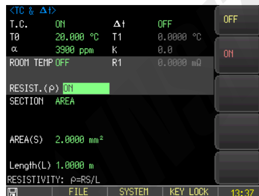
Figure 6- 4 Resistivity cross-section shape-area
