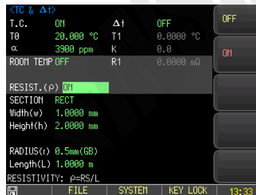
Figure 6- 2 Resistivity cross-section shape- -a rectangle
