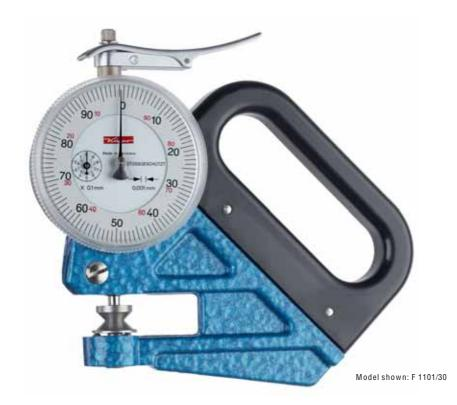
These handy instruments are used exclusively to measure the thickness of thin foils. The frame has the required rigidity, the insulation of the handle prevents transfer of heat from the hand of the user to the sensitive mechanical parts of the Dial Gauge.
