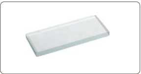
50mm reading scale (check magnification accuracy)
