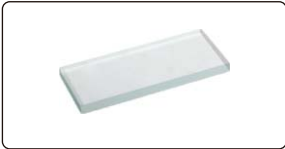
50mm reading scale (check magnification accuracy)
