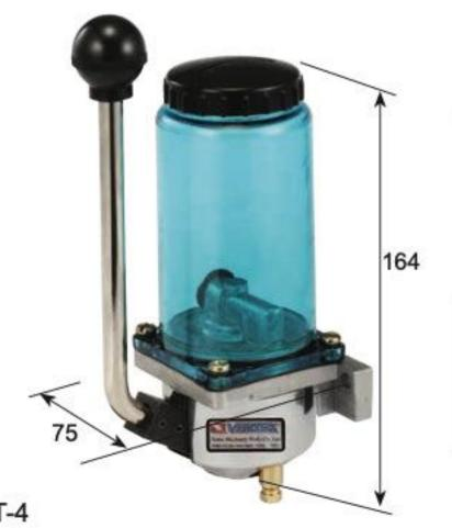
Rattling hand pump LT model Rattle the lever of the pump reiteratively and the oil will be pressured into the main pipe. When the lever is released, it will return to the original position automatically.
