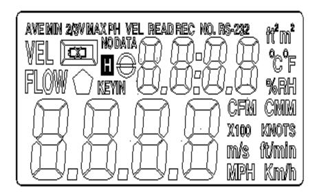
AVE: When method of average is selected by OPTION button for flow measurement, this symbol will appears.
