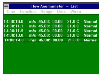
If this option is selected or CTRL+L is pressed, a window, which lists the date, function, range, and value every sampling, shall appear on the screen.
