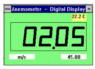
If this option is selected or CTRL+D are pressed, a window, which emulates multimeter's LCD display, shall appear on the screen.
