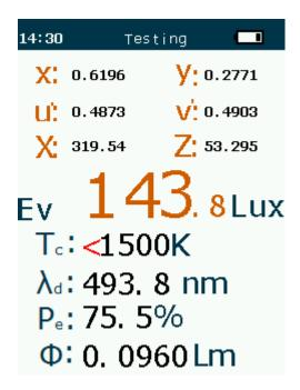
When a device complete a set of data testing, user can press 'MENU' key to jump into homepage and perform other operations. If press 'MENU' again, the page would return to measuring page.
