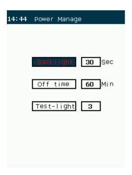
There are functions include screen backlighting time setting, auto-shut off time setting and backlight brightness adjustment.
