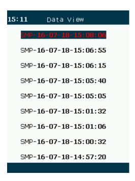
Data list is sorted by time, and device only stores latest nine dada. New data would cover previous data automatically.
