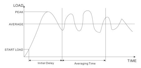
**MOD2:** This function calculates the average above the set minimum measured value. When the measured value falls below the set minimum value again, the measurement is finished. This measuring procedure is possible over a period of 10 minutes. As long as the measuring time of 10 minutes is not exceeded, this measurement can be resumed at any time.
