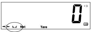
In case that the scales do not react, check the power supply of the display. If the sign for stable operation does not appear, check the subsurface and align the scales.
