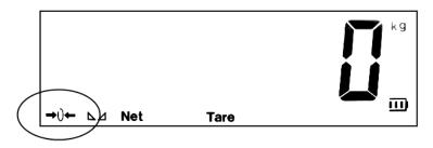
If you want to display the present weight after starting the scales (useful for container weighing), you need to change some items in the menu screen. Refer to the menu mode C07 / C08 / C09 as well as C05 to determine the internal zero position.
