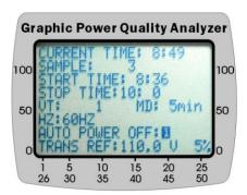
**TRANSIENT REFERENCE:** set the nominal voltage and threshold (%) for transient capture.
