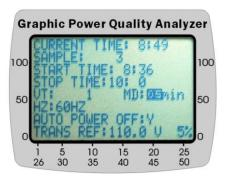
**HZ:** set the operating frequency to 50Hz, 60Hz, or Auto.
