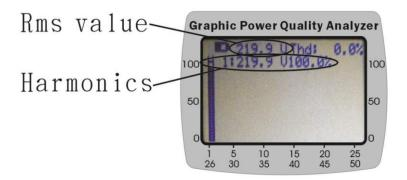
%THD-F: Total Harmonic Distortion with respect to Fundamental frequency %THD-F = ( $\sqrt{(V2^2+V3^2+...+V49^2+V50^2)}$ ) / V1) \* 100
