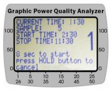
Users always have 8 seconds to cancel datalogging by pressing the HOLD button for **about 2 seconds**. If users do not press HOLD/CANCEL button, the unit starts datalogging, and **the LED at the bottom starts blinking**.
