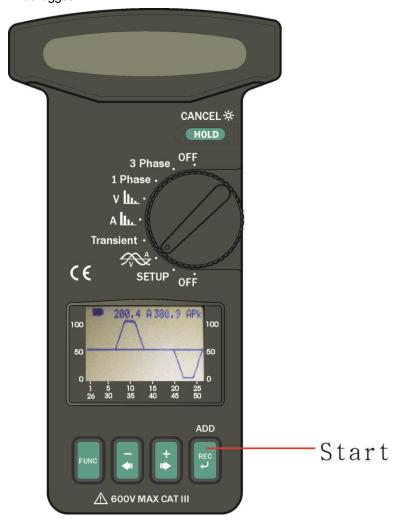
**NOTE:** Users can specify how many points per cycle to be logged in the WAVEFORM CONFIGURATION of SETUP.
