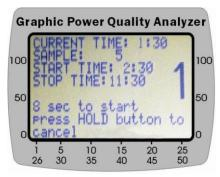
Users always have 8 seconds to cancel Datalogging by pressing the HOLD button for **about 2 seconds**. If users do not press HOLD/CANCEL button, the unit starts Datalogging, and <u>the LED next to the REC button starts blinking</u>.
