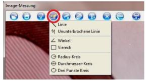
Perform measurements after calibrating the microscope. Choose a suitable object and mark the measuring points in the image. The measurement result is displayed. By clicking the mouse in the result, the image can be drawn.
