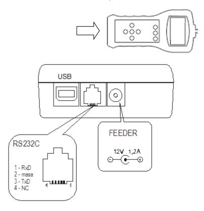
On the bottom of the forge gauge you can find an USB and a RS-232C interface, as well as a connector for power supply.
