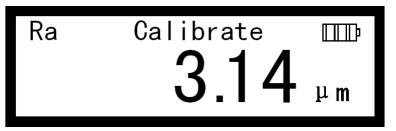
Put the instrument in the scribed line area. Sensor taxiing direction perpendicular to the scribed line of texture direction. Press the Start Key to exit the status of Calibration. Repeated calibration could improve precision.
