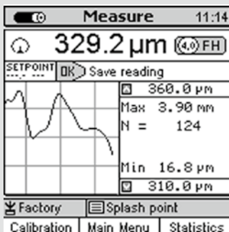
Measuring Value combined with Real-Time Trend Diagram
