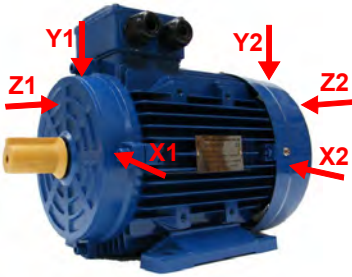
Figure 11: Measuring Points on Electric Motors
