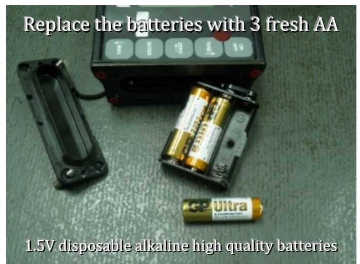
being careful not to damage the wiring
