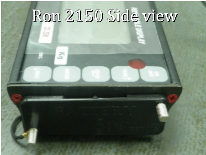
Unscrew the two screws on the side of the indicator
