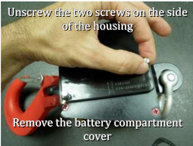
Gently remove the battery holder
