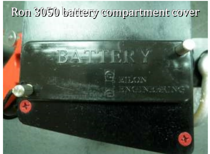
The screws should remain securely inside of the lid
