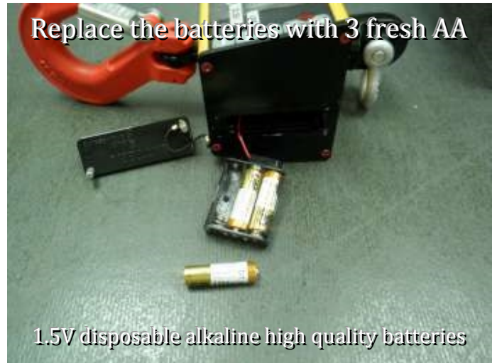
Gently remove the battery holder
