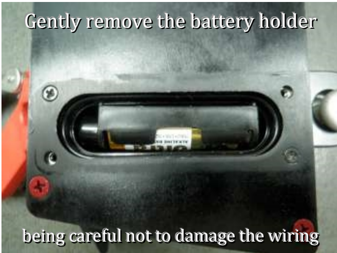
Remove the battery compartment cover
