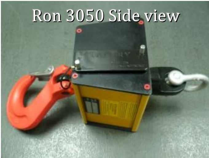
Unscrew the two screws on the side of the housing
