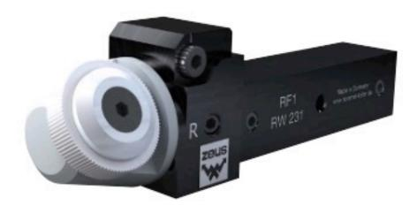
Knurl profile at workpiece (DIN 82)
