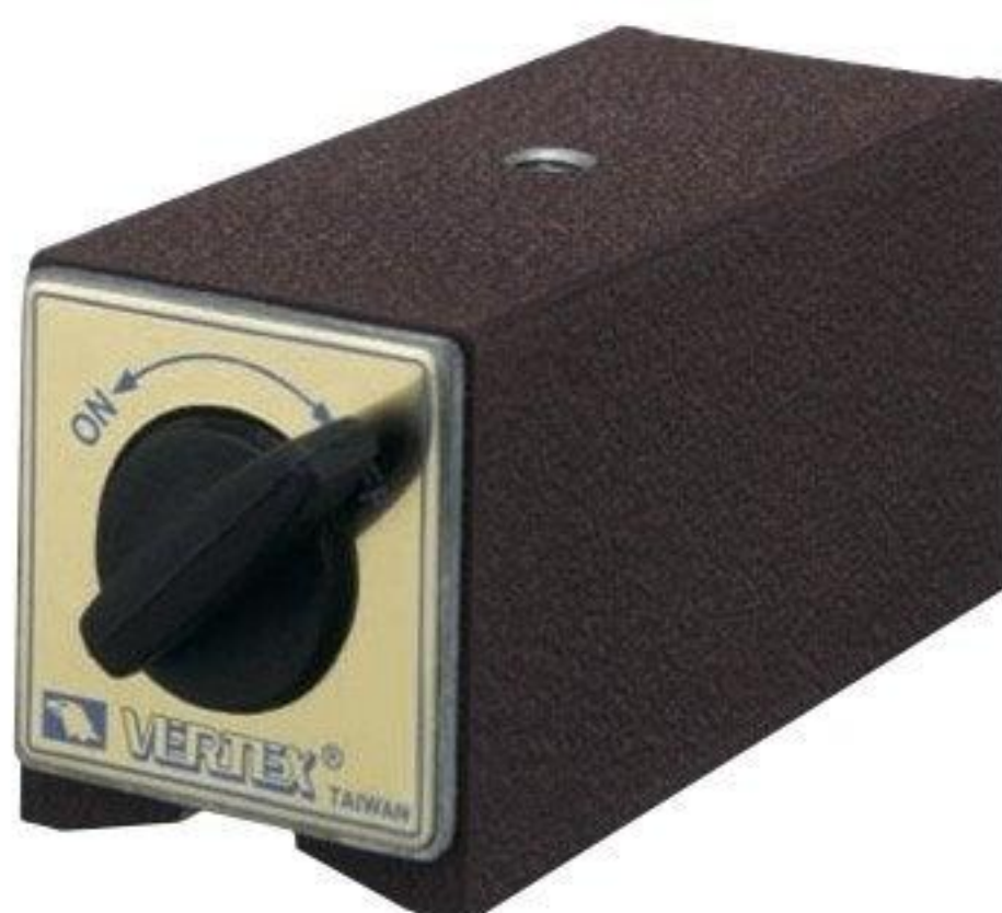
ORDER NO. VMB-11 MAGNETIC BASE ONLY M8X1.25p,140kgs
