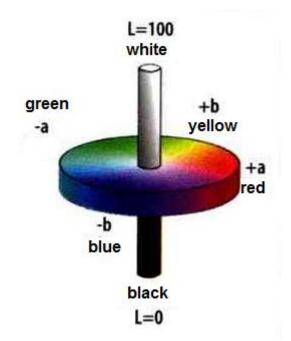
Here you can see the colour space  $L^*a^*b$ . This colour space covers all colors that are visible with the naked eye. L=100 stands for white and L=0 for black. "a+" and "a-" or "b+" and "b-" stands for the colour contrasts red, green, yellow and blue.
