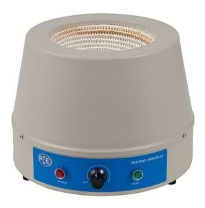
HeatingMantle for 2000 ml round-bottom flask / stepless variable (rotaryswitch) / with 450 watt power / with integrated controller / temperature range 0... 450 °C
