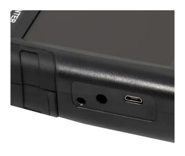
Air sampler for indicative measurement / Adjustable alarm limits / Data logger / Micro USB **charging** interface / Measuring range 0 ... 1000  $\mu$ g/m³ / Mass concentration / Approx. 9 hours of battery life / 3.2" color display / Carrying case / 1/4" tripod connection
