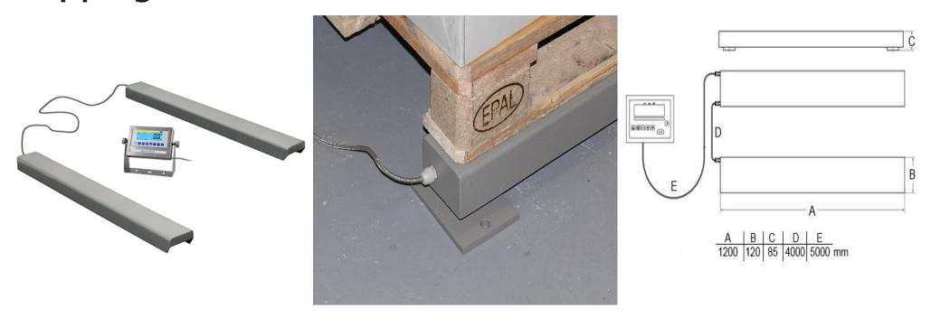
PCE-SW 5000N is a portable battery-powered industrial pallet scale or floor scale featuring two heavy-duty parallel weighing beams made of lacquered steel that can be positioned up to 4 m / 13 ft apart. Thus, the adjustable width accommodates multiple pallet, box and container sizes. In addition, the scale's stainless-steel-encased display can be placed up to 4 m / 13 ft away from the weighing beams, allowing for wall mounting.
