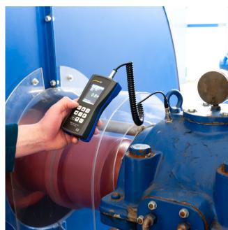
Handy entry-level device for vibration monitoring of machines and systems / HOLD function / Peak value measurement / Handheld device for mobile vibration measurement / Automatic ISO 10816-3 evaluation
