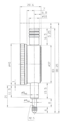
On request the Safety Dial Gauges SI-45 and SI-45/0.8 can also be supplied as waterproof version. Their model designations are SI-45 W and SI-45/0.8 W. Please note that in this case the dimensions of the above drawing do not apply.
