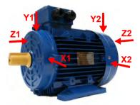
Figure 11: Measuring Points on Electric Motors
