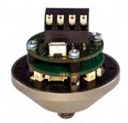
Figure 1: Open PCE-VS11 with terminals for power supply / relay output and USB socket
