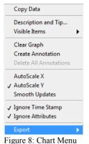
By right clicking on the chart area you can automatically scale the chart (auto scaling Y). Double-clicking on the scale label of the Y-axis allows you to manually rescale the axis by overwriting it.
