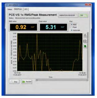
Figure 4: RMS /Peak Measurement
